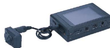
Connected /w the PVR via the attached Cable
