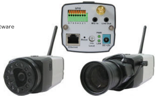
CS Mount IR Lens, f 6mm / F1.8
